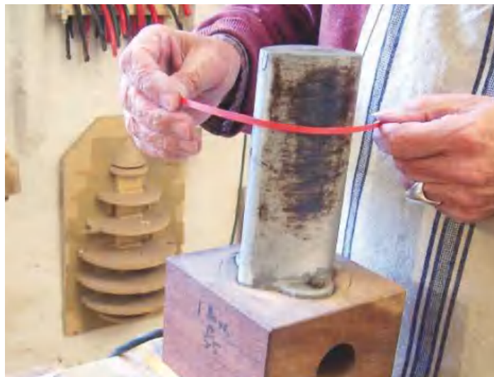
STEP 4. Bending the veneer strips on the hot iron
